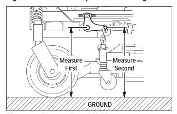
Figure 38. Measure Front Lift Pivot
